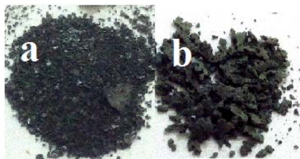
Fig. 1: a. MoS 2 sample, b. Mo-W-S sample
